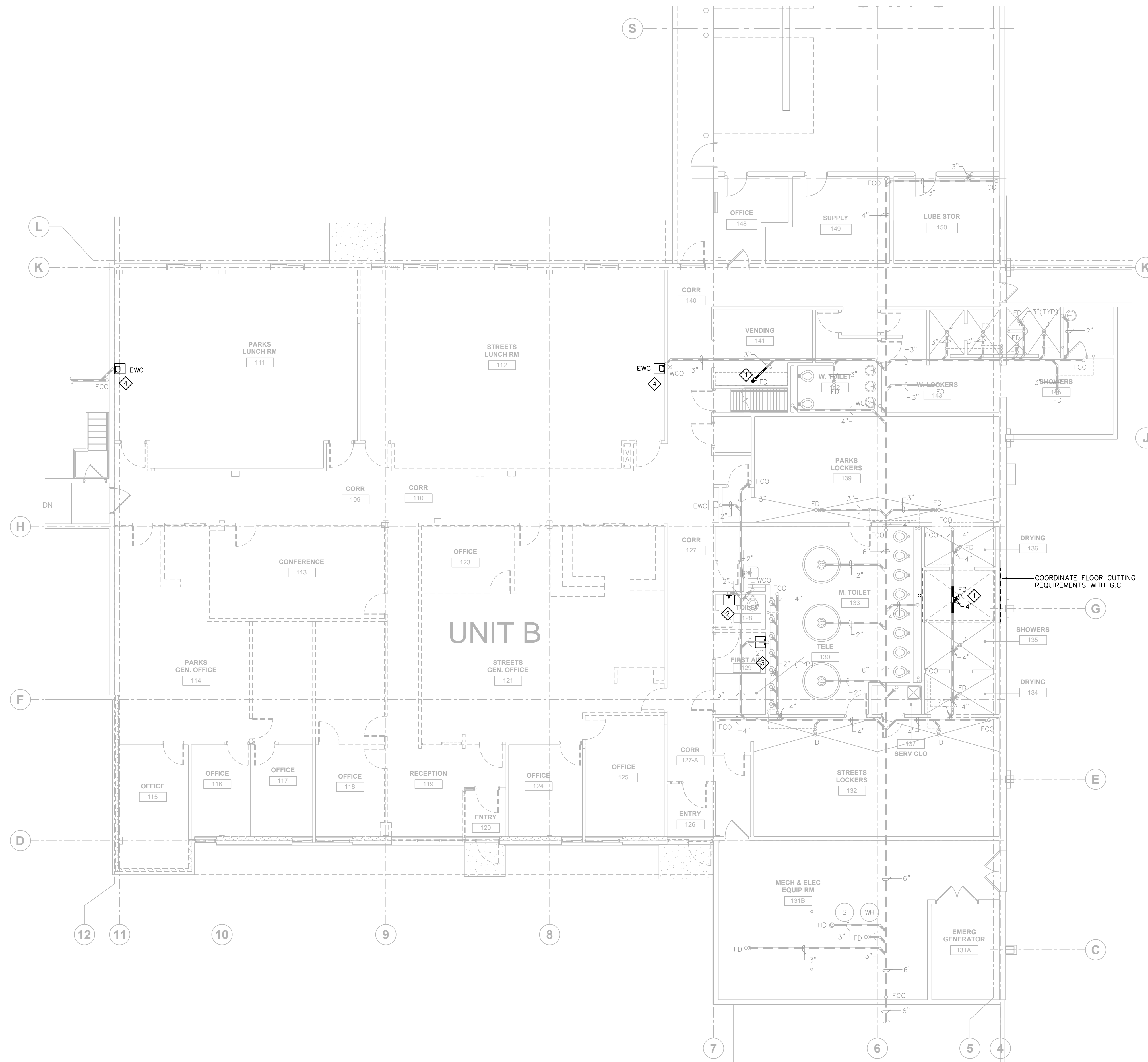
1 UNIT B - UNDERGROUND PLUMBING DEMOLITION PLAN 1/8" = 1'-0"
